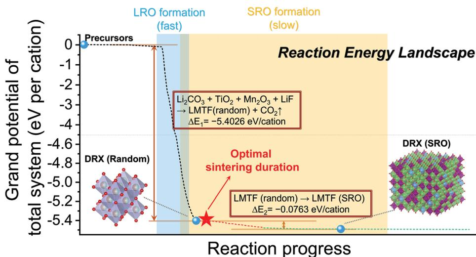
**Figure 3.** Schematic of the reaction energy in the LMTF synthesis process. The grand potential evolution of the total system is computed ab initio for the random rock salt and the short-range ordered rock salt (simulated at 1273 K), and schematically interpolated (with dashed line). Note that two different energy scales are used (separated at  $-4.5$  eV) to highlight the small energy decrease in the SRO formation.
