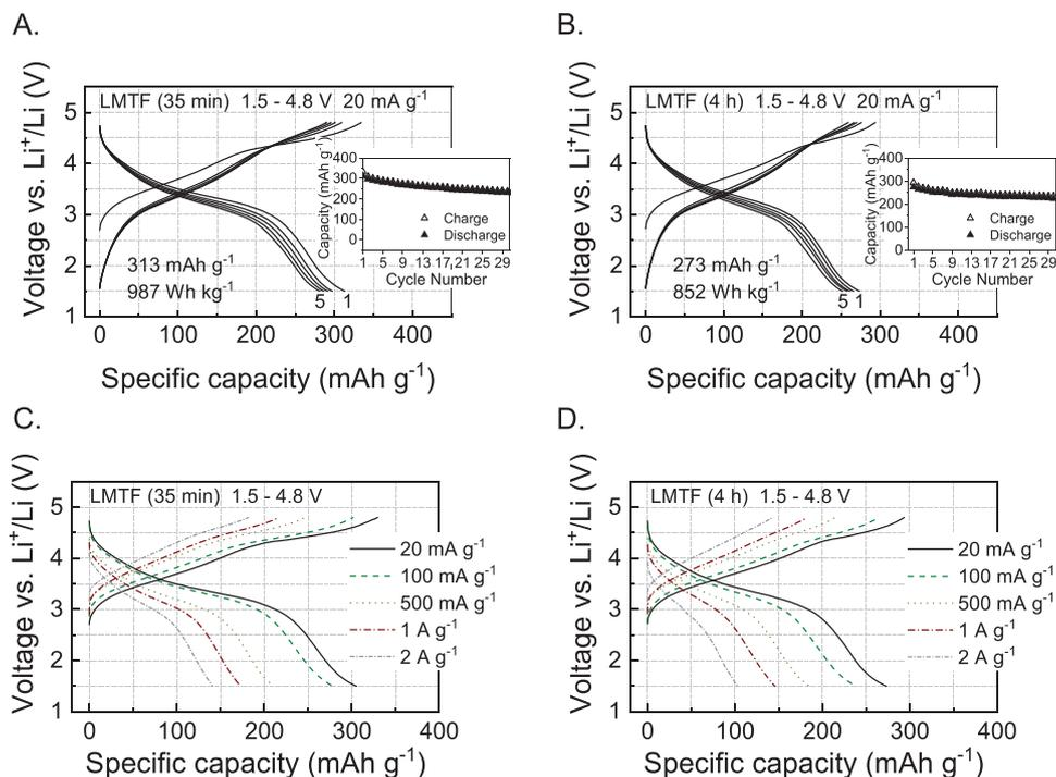
**Figure 4.** Electrochemical performance of LMTF (35 min) and LMTF (4 h). Voltage profiles and capacity retention of A) LMTF (35 min) and B) LMTF (4 h) within the voltage window of 1.5–4.8 V at 20 mA g<sup>-1</sup> and 25 °C. Rate capability of C) LMTF (35 min) and D) LMTF (4 h): the first-cycle voltage profiles when cycled between 1.5 and 4.8 V at 20, 100, 500, 1000, and 2000 mA g<sup>-1</sup>.
